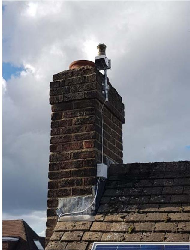
Here's a photo of the FRIPON camera installed on my (now fire-free) chimney, with uninterrupted views of East Barnet and the English sky. An Ethernet cable connects it to its own dedicated Dell PC and a power-over-internet power injector. So far so good – now for the software.
